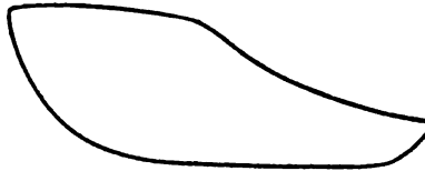
Fig. 257. Indicator Card with Exhaust Lap too large.
